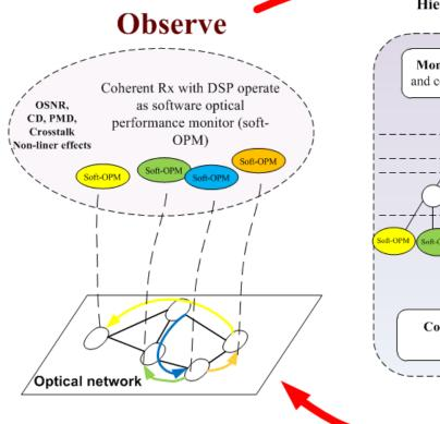
Hierarchical Monitoring and **Control plane** Monitoring plane: Transfer, filter, and correlate monitoring information . . . ... Soft-OPM Soft-OPN Soft-OP Control plane: apply network configuration changes
