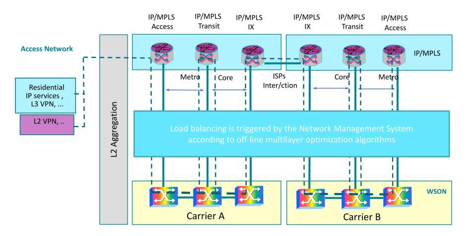
Load balancing between IP/MPLS and optical. High capacity flows (e.g between IP access and IP interconnection) are directly transported over optical
