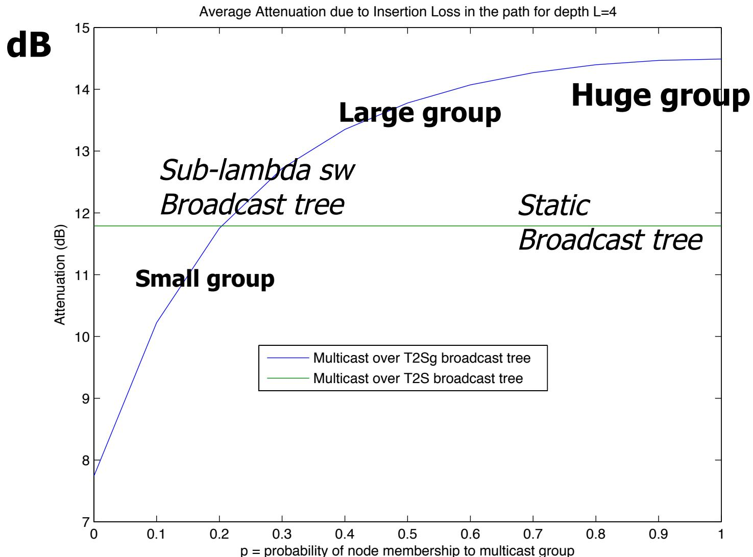
Fig. 13. Average attenuation due to insertion loss in a path root-leaf for a 4-node-deep binary light-tree
