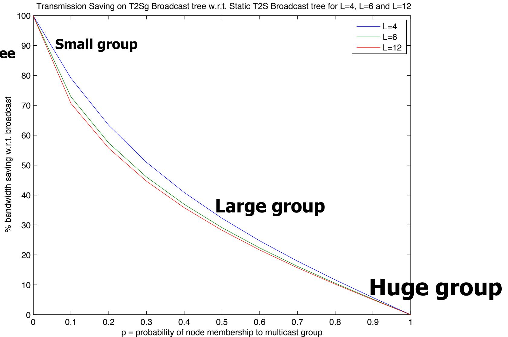
Fig. 12. Relative bandwidth saving featured by T2Sg with respect to T2S in a shared broadcast tree
