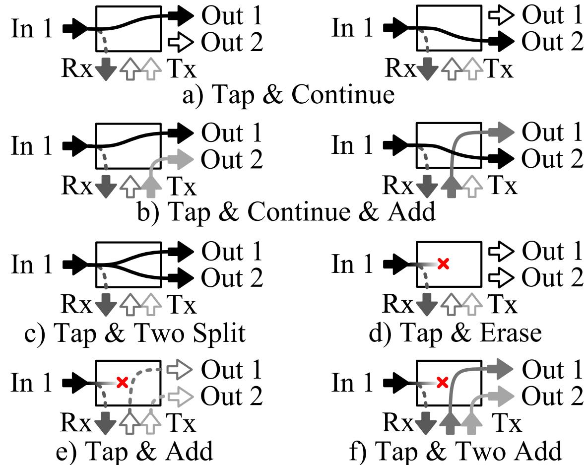
Fig. 2. T2Sg Switch functionalities
