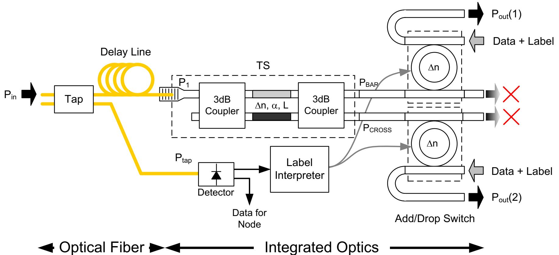
Fig. 3. Structure of the proposed Tap 2-Split Traffic Grooming Switch (T2Sg).
