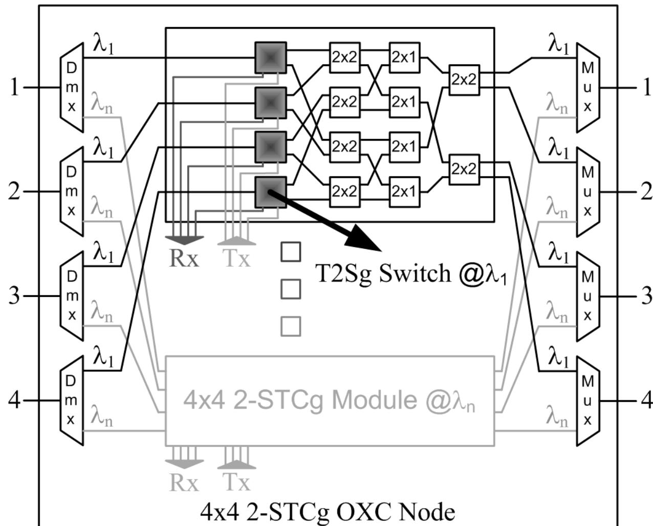
Fig. 1. 4x4 2-STCg OXC node structure.
