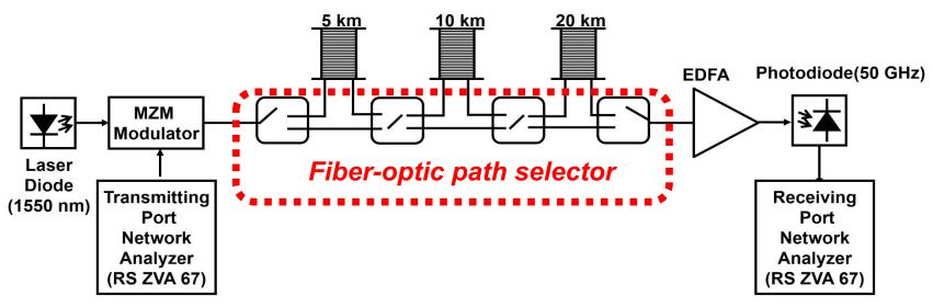
Experimental setup is composed of Vector Network Analyzer, DFB Laser, Mach Zehnder Modulator, fiber-optic link (5 km, 10 km, 15 km, 20 km, 25 km, 30 km and 35 km) and photodiode.
