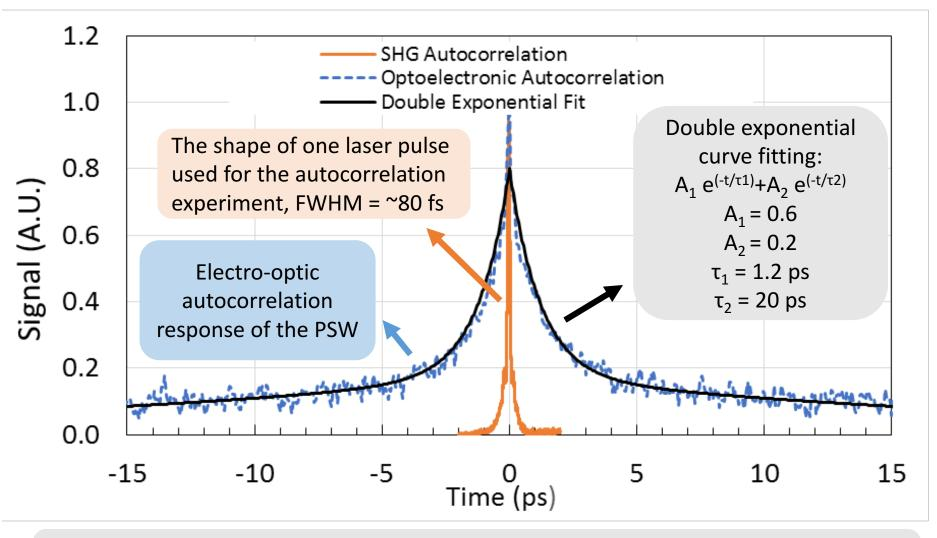
The measured ultra-fast **1.2 ps response time** makes the switch available to have sampling rates (laser pulse repetition rates) up to 100 GHz.
