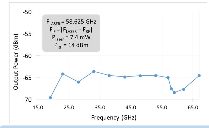
The mixing loss around 80 dB, is in the same order of magnitude as unbiased UTC photodiodes used as mixers
