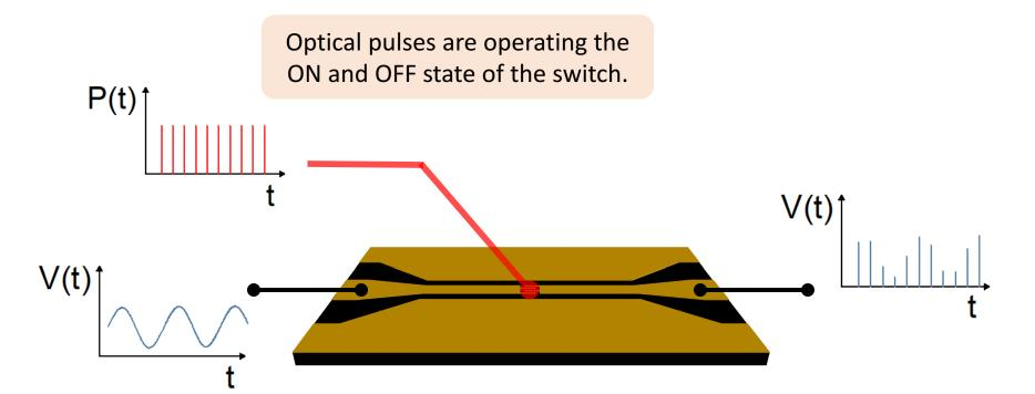
The input of the switch is an analog high-frequency electrical signal.
