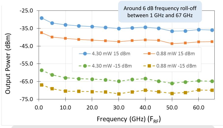
The low variation of output power confirms the wide electrical bandwidth of the PSW
